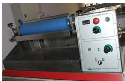
a. Padding machine for textile impregnation with polymeric and functionalization substances (ROACHES, UK)
