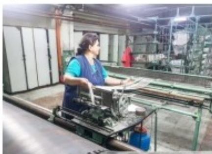
Fig. 1. Operatia de urzit in benzi
