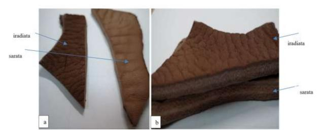
Figure 3. Crust leather obtained by vegetable tanning of the hides, preservation by salting and by gamma irradiation a) grain and b) section
